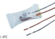
KSD-4001 OPEN:8°C CLOSE:-7°C+FUSE72°C
