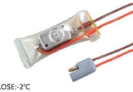
KSD-2011 OPEN:13°C CLOSE:-4°C+FUSE72°C
