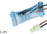
KSD-2011 OPEN:13°C CLOSE:-4°C+FUSE72°C
