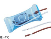
KSD-2003 OPEN:12°C CLOSE:-5°C+FUSE72°C
