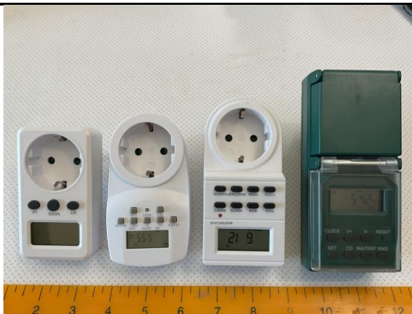
Sample Description: Electronic plug-in time switch, Direct plug-in power meter Model No.: TS-ED204, TS-ED1-2, TS-ED201-16, TS-JD01
