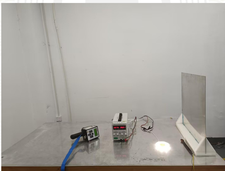
Figure 4: Electrostatic Discharge Test Setup
