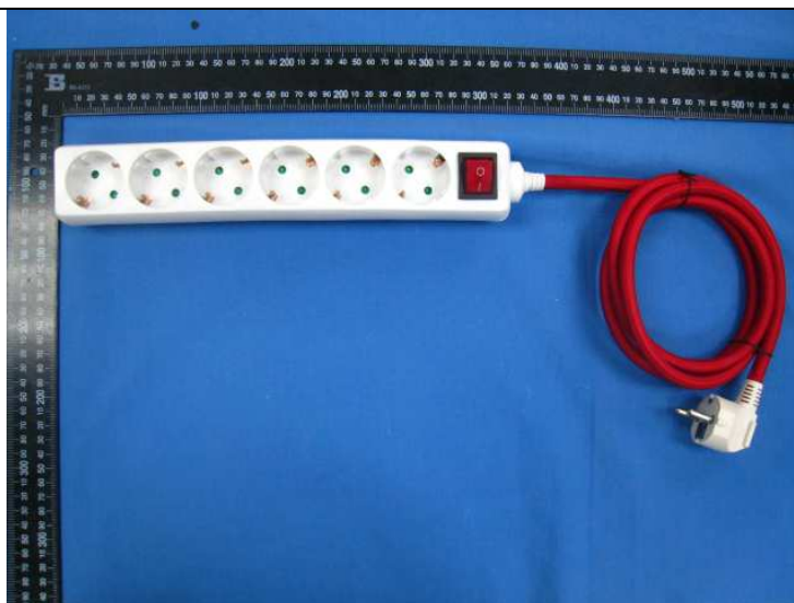
Front view of 106BK with additional fabric braided cover over the cable
