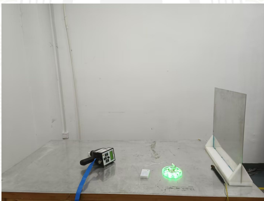
Figure 4: Electrostatic Discharge Test Setup
